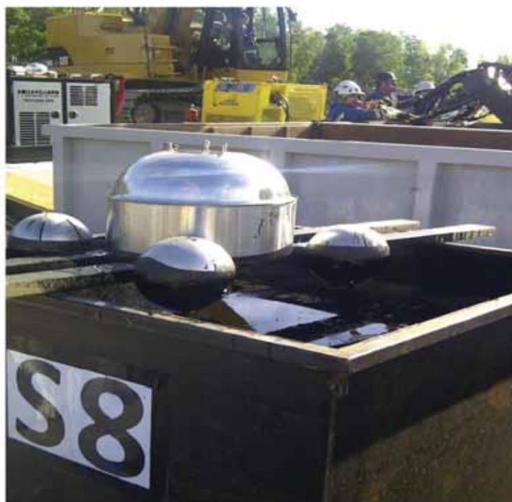
Figure 2: Floating flux chamber suspended above oil spill after sampling event
