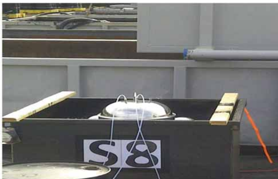
Figure 1: Floating flux chamber in sampling position on oil spill in Tank S8
