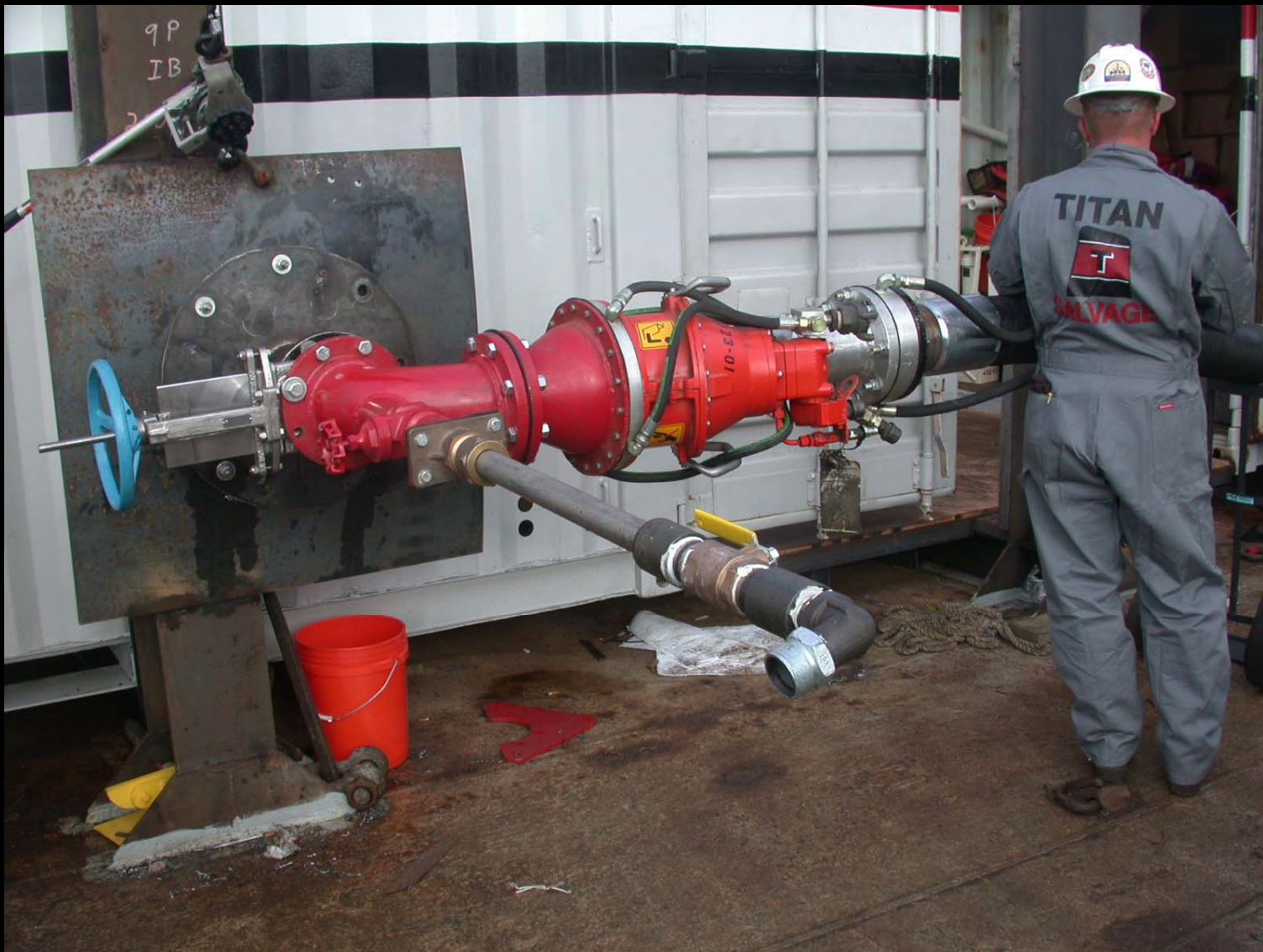
THE REAL THING, VOPS SYSTEM PUMP ARRANGEMENT
