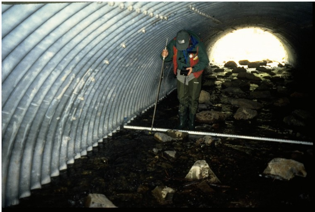
Figure 8. Conducting Velocity Measurements on a Cross Section in a Natural Bottom Culvert. Source: George Robison
