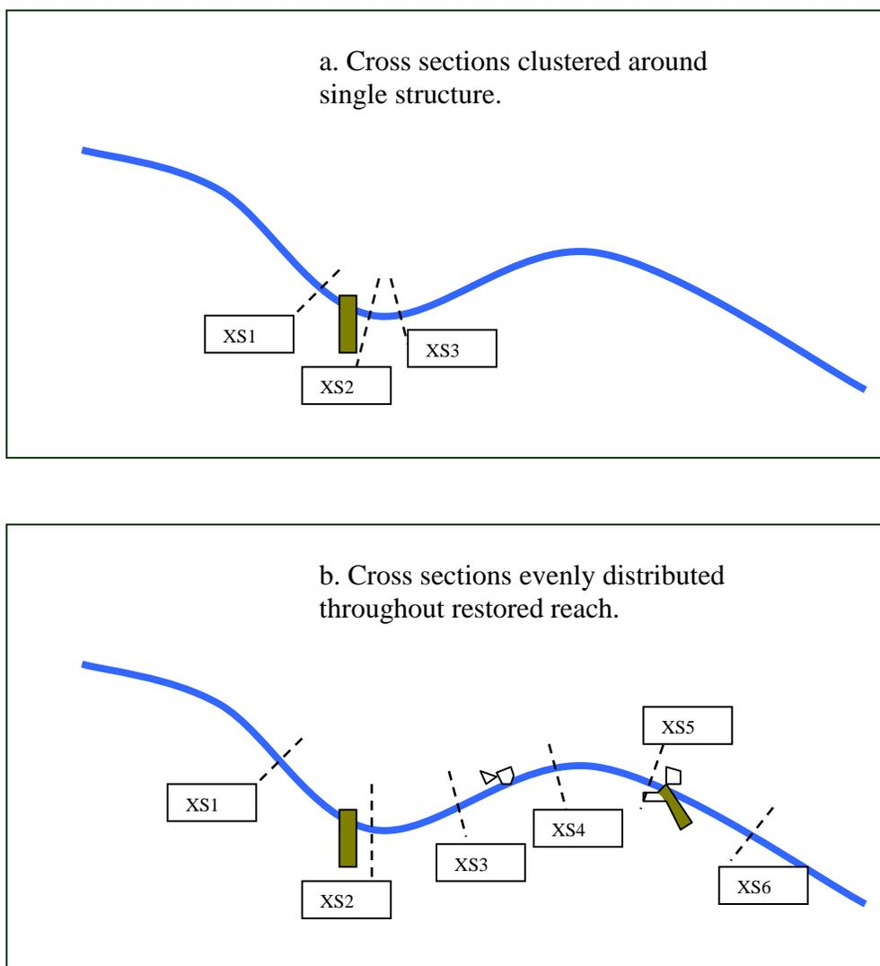
**Figure 4.** Cross Section Locations for Individual Structures and Stream Reaches.
