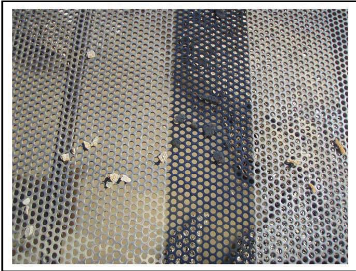
3/8 in Diameter Punch-Holed Steel Plate
