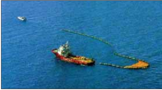
Mechanical recovery off-shore, NOFO-oil-on-water exercise
