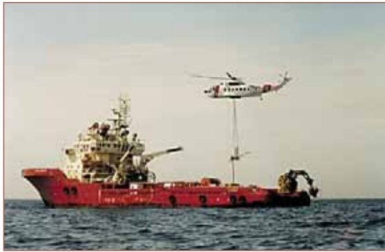
The Norwegian developed Heli-bucket, Response 3000, filling dispersant from supply vessel.
