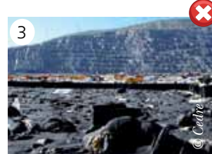
Intermediate storage sites: 1) pastes and liquid waste in a pit 2) solid waste in skips 3) unacceptable mixture of solid, paste and liquid waste in the same pit.
