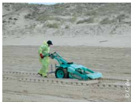
Mechanical selective sand screening
