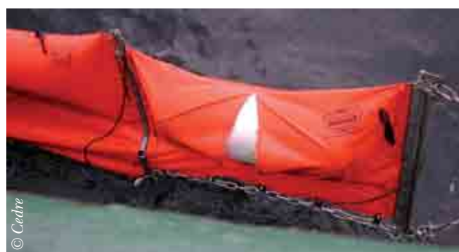
A tear caused when towing an inflatable boom, due to excessive towing strain
