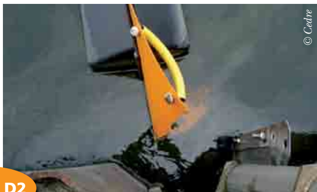
Boom ripped away from a tidal compensator
