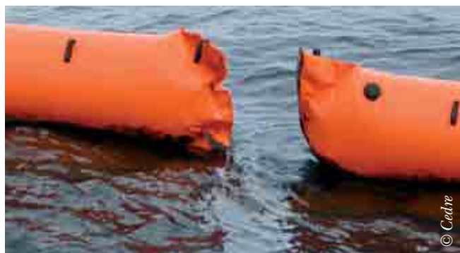
Breaking away of boom sections at a connection during recovery operations at sea (Prestige spill, Spain)
