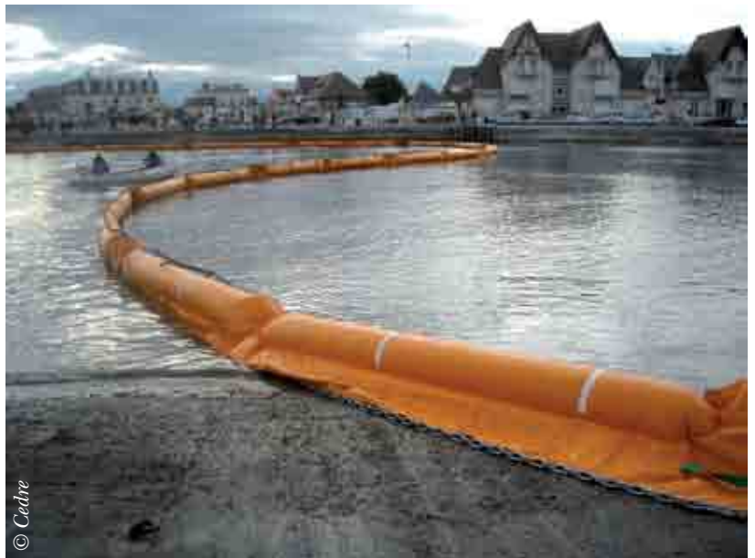
Deploying an inflatable curtain boom
