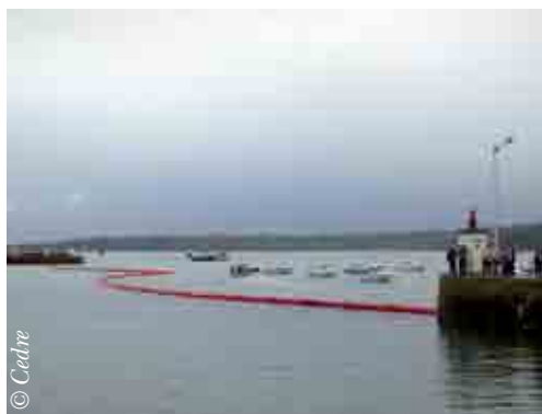
Deploying an inflatable boom between two walls at a harbour entrance
