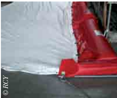
Maritime operations boom: view of the geotextile skirt
