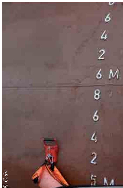
Magnetic anchor on a ship's hull
