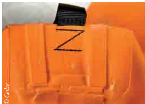
Pieces of fabric joined together by heat sealing
