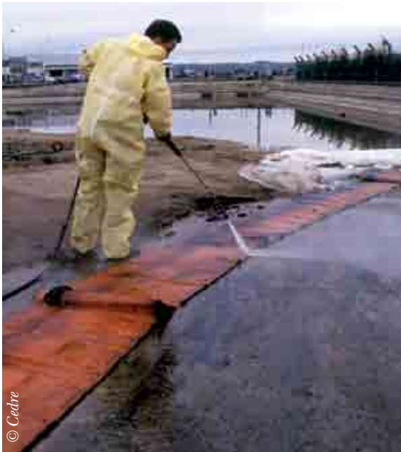
High pressure washing of a spill response boom
