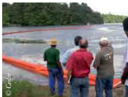
Deploying an inflatable boom across a river
