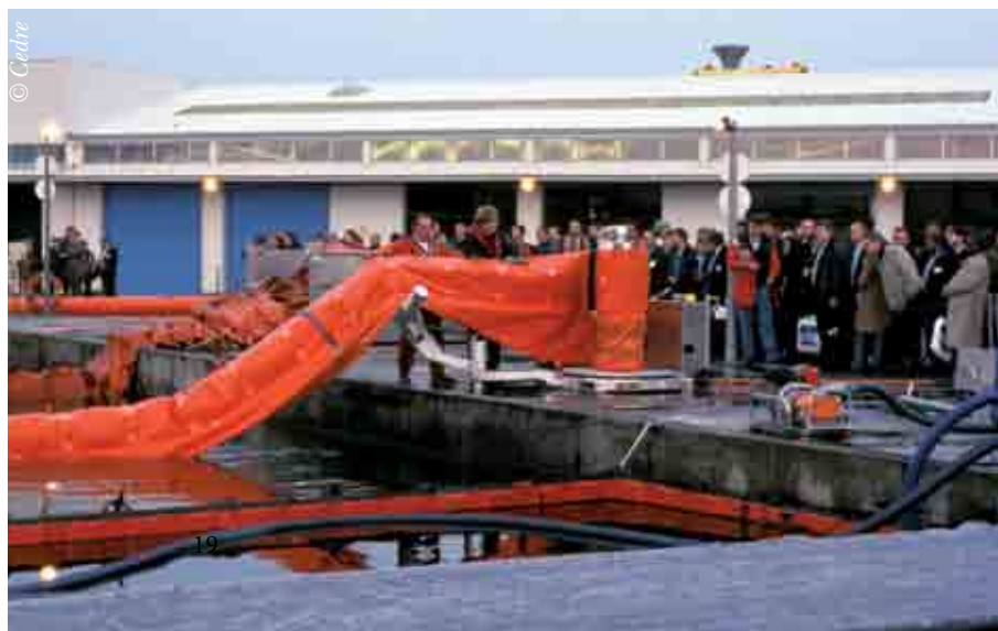
Deploying a self-inflating boom
