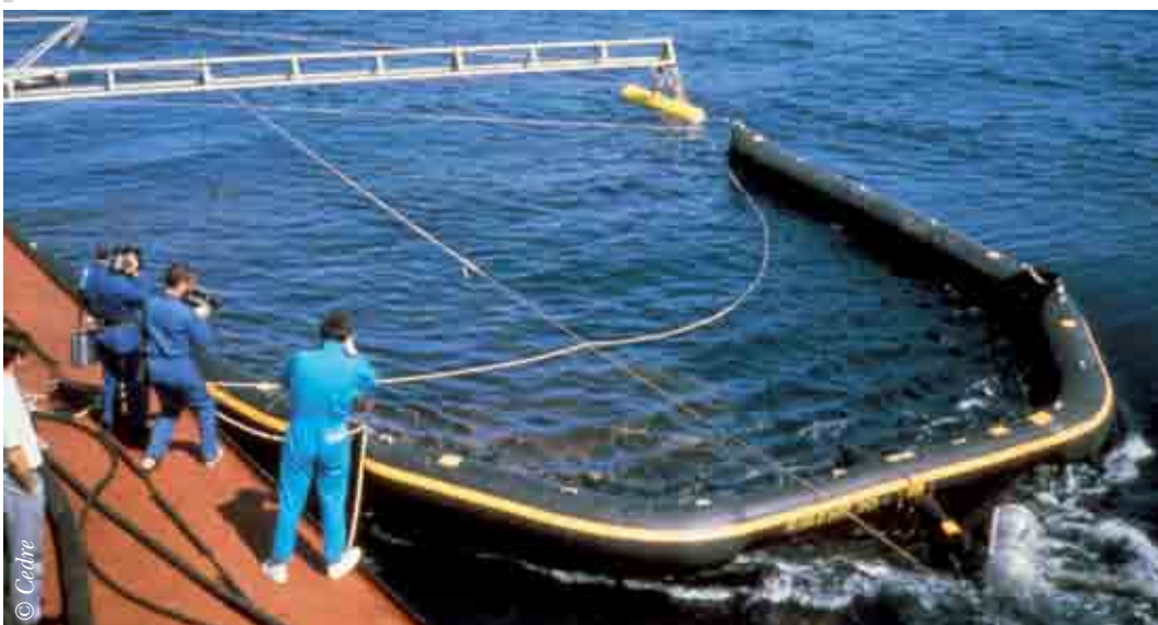
Boom attached to an outrigger and comprising a recovery system, deployed from a single vessel
