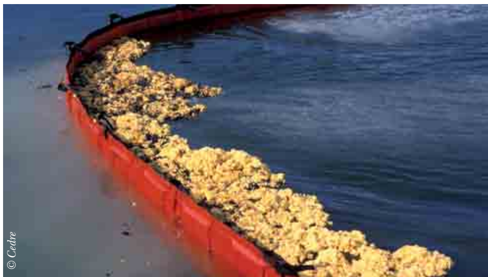
Containment of oiled loose sorbents by a foam-filled fence boom
