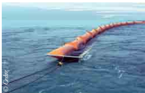
Towing an inflatable boom
