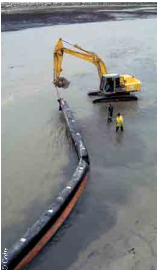
Deploying a boom using earthmoving equipment
