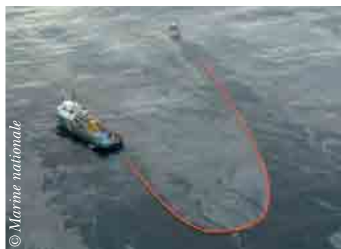
Setting up a boom in a J-configuration, CMA CGM Strauss spill, 2010
