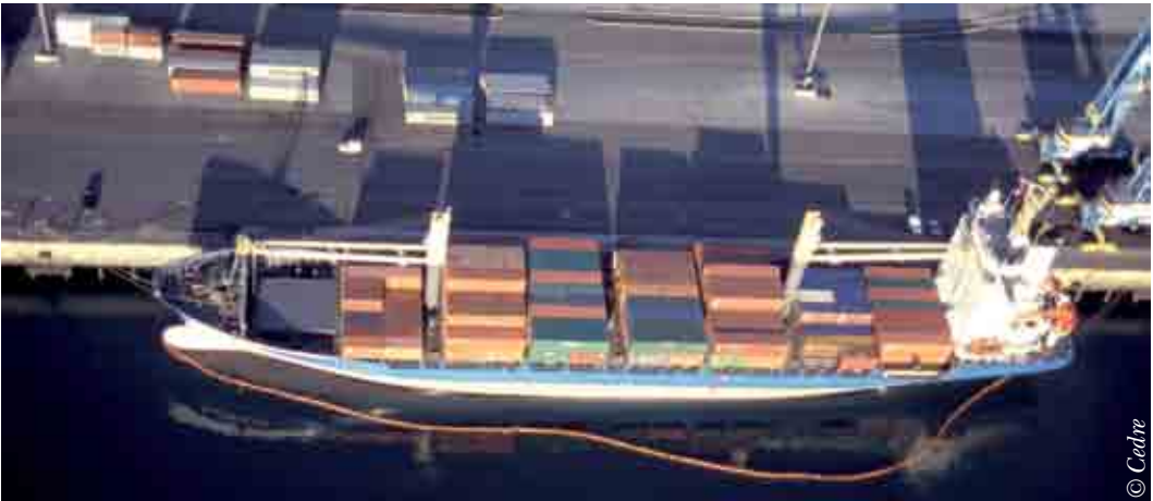
Spill response boom set up to contain any leaks, Melbridge Bilbao, 2001
