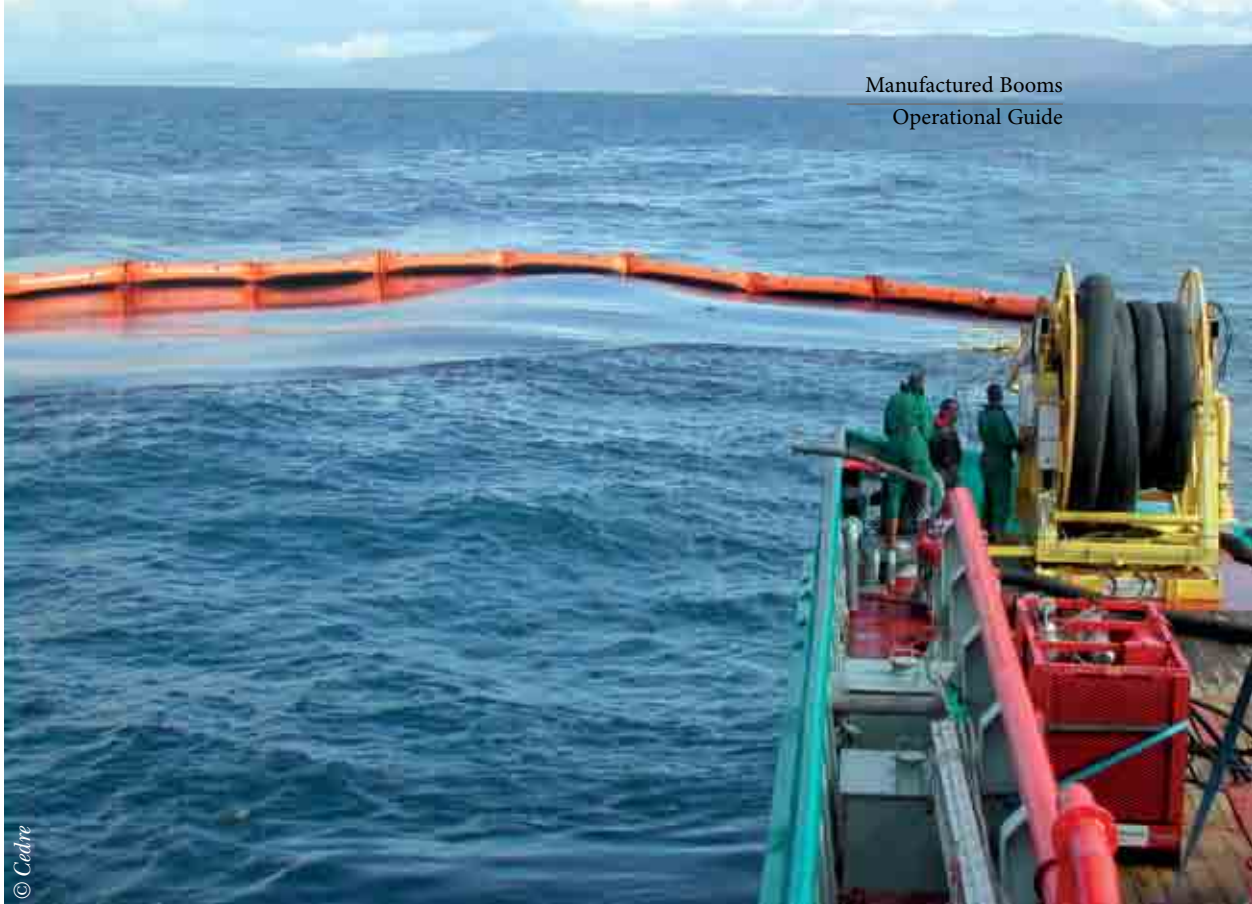
Recovering a contained slick using an inflatable boom from the BSAD Ailette, Prestige, 2002
