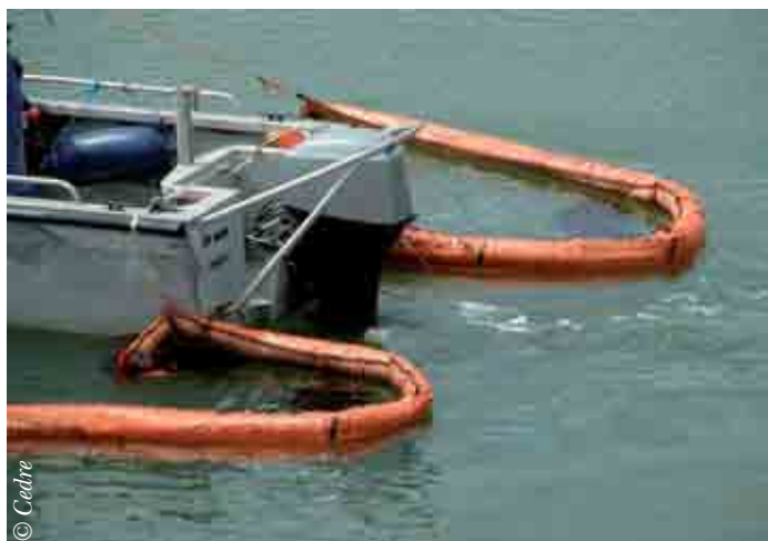
Testing a sorbent boom with a ballasted skirt
