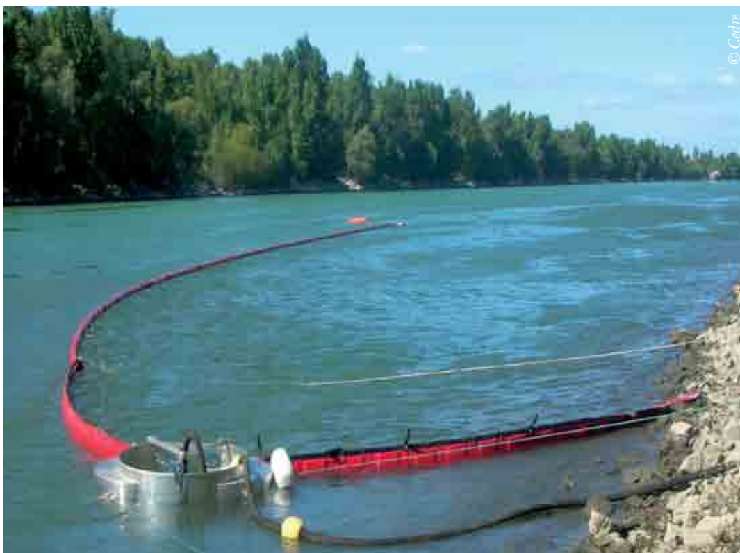
Boom deployment using a paravane and associated recovery system
