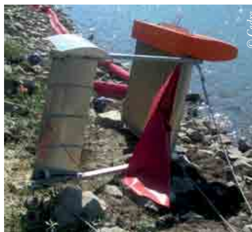
Close-up of a paravane on a bank before being deployed
