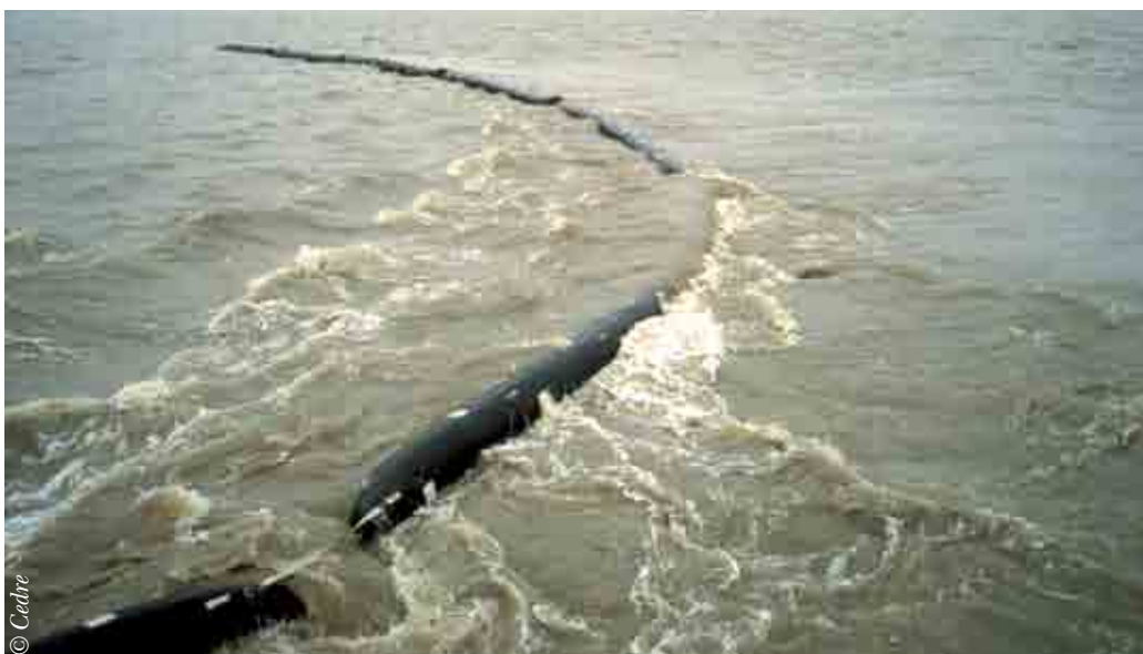
Boom failure due to currents
