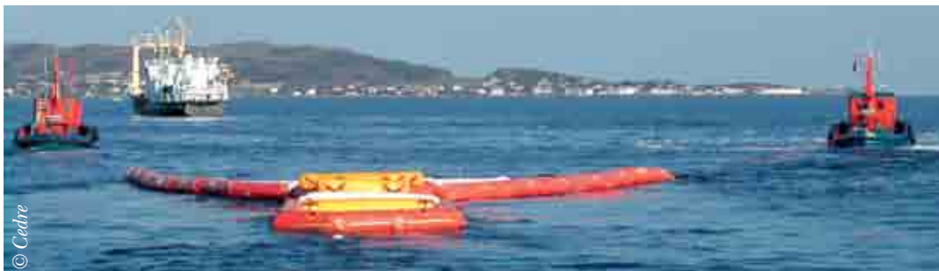
Trawl boom towed by two vessels
