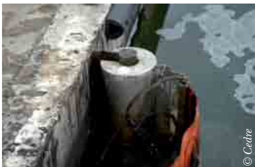
Sliding cylindrical float on permanent rail
