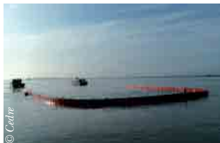
Boom in a U-configuration towed by a pair of vessels
