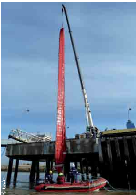
Retrieving a fence boom from a wharf following deployment
