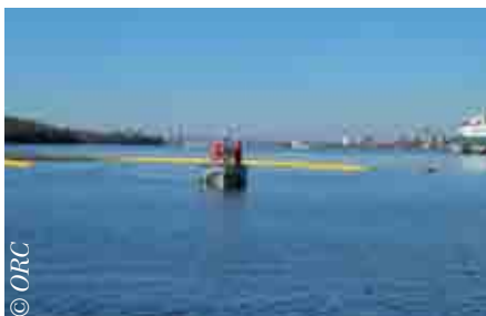
Towing a boom in a U-configuration using a boat and a paravane
