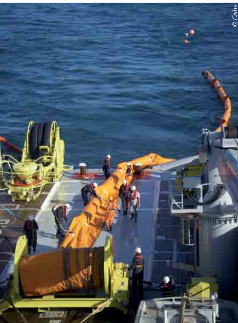
Deploying an inflatable curtain boom
