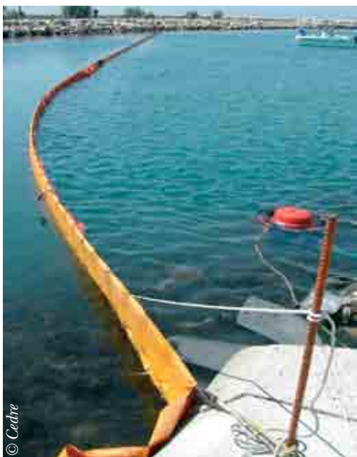
Deploying a foam-filled fence boom to close off a harbour entrance
