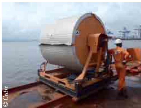
Sheet metal protecting a boom stored on a reel against severe weather and rodents
