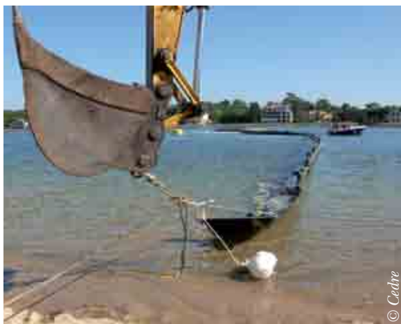
Using a power shovel to help deploy a boom
