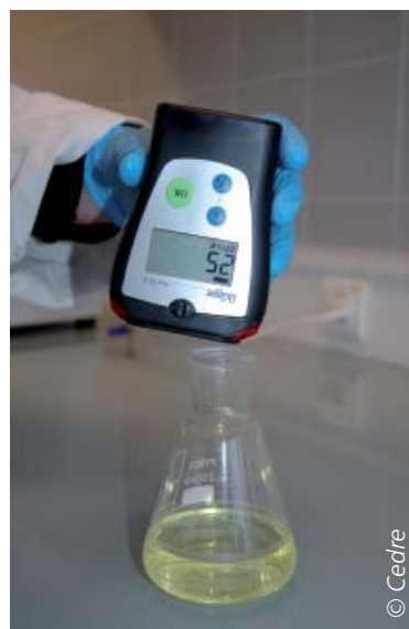
Measuring vapours using an explosimeter.
