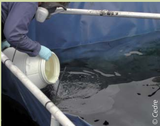
Simulation of an unleaded gasoline spill in a floating cell
