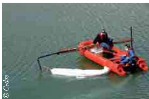
Unilateral towing of a boom made of polypropylene fibres
