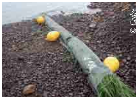
Barrier made of mesh and vegetation with buoys for increased buoyancy
