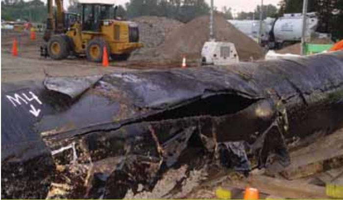
Section of pipe from Kalamazoo spill containing rupture. Rupture length is approx 6 ft 5 inches and is 4 1/2 inches wide at the widest location.
