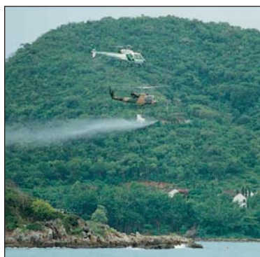
Building in realism: in this oil spill exercise, the application of dispersants is simulated using vegetable colouring as a substitute for the real thing.
