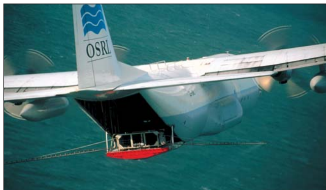
Dispersant application options are discussed, including boat-based systems, fixed wing aircraft-based systems (above), and helicopter-based systems.
