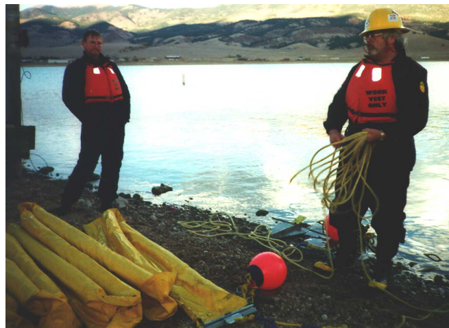
Figure 8-10. Boom faked out in zigzag with anchor attached.
