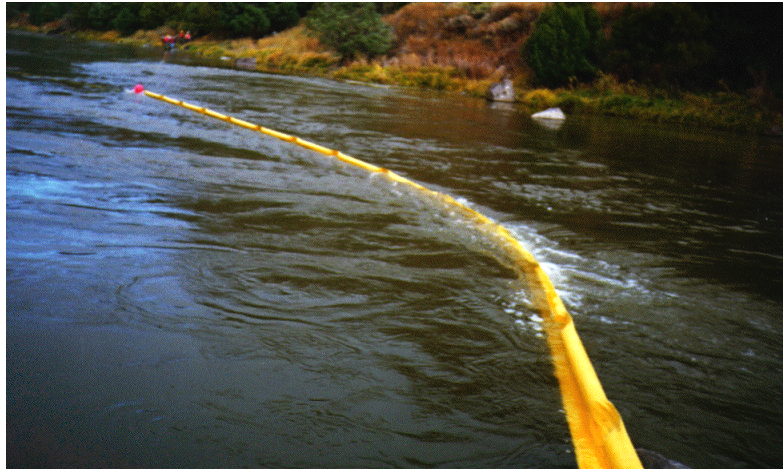
Figure 3-3. Boom submergence failure in swift current.
