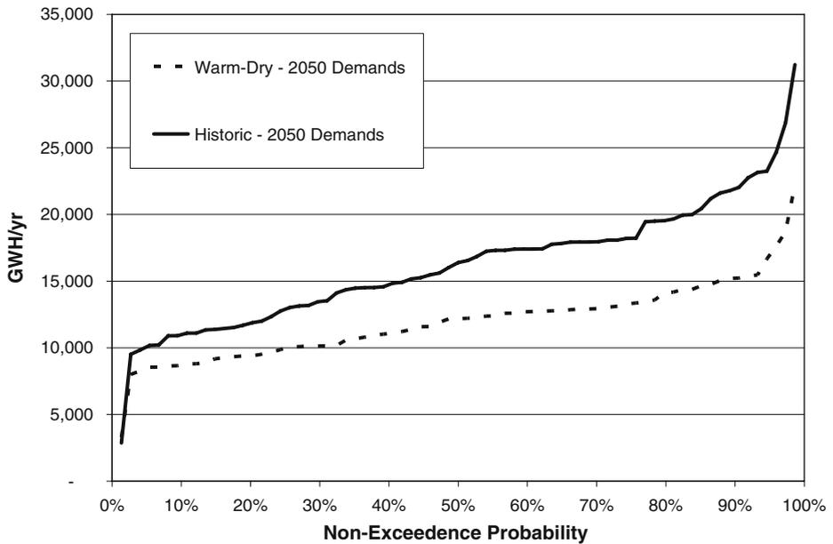
**Fig. 3** Frequency of annual power generation from major water supply reservoirs (based on 72 years). Under dry-warm hydrology annual average hydropower production is less variable, due to reduced flows and storage
