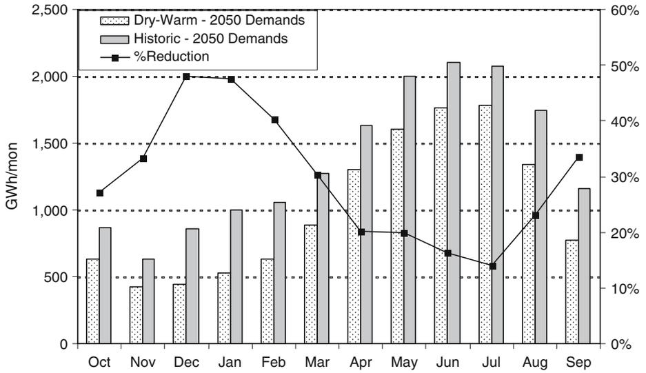
**Fig. 2** Average monthly power generation and percent reduction in generation (dry warm vs. historical hydrology). Whereas power generation is always lower under the dry-warm climate, reduction is the greatest for the low-generation months (Nov–Feb), based on a 72-year monthly time span
