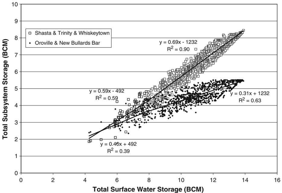
**Fig. 8** Surface water storage allocation for major reservoir sub-systems in the Sacramento Valley (historical climate based on 72 years). For the Oroville-New Bullards Bar Subsystem a change in storage rate is more evident after 8 BCM
