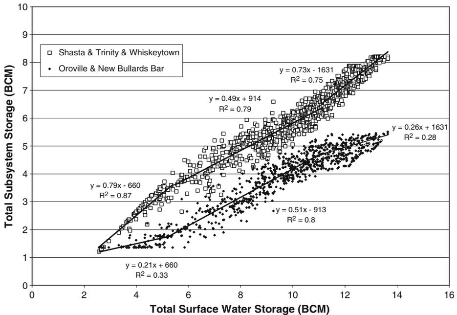
**Fig. 9** Surface water storage allocation for major reservoir sub-systems in the Sacramento Valley (dry climate warming based on 72-years). Storage rates display statistically significant ( $p$  value  $<0.01$ ) changes at 5.4 and 11.1 BCM
