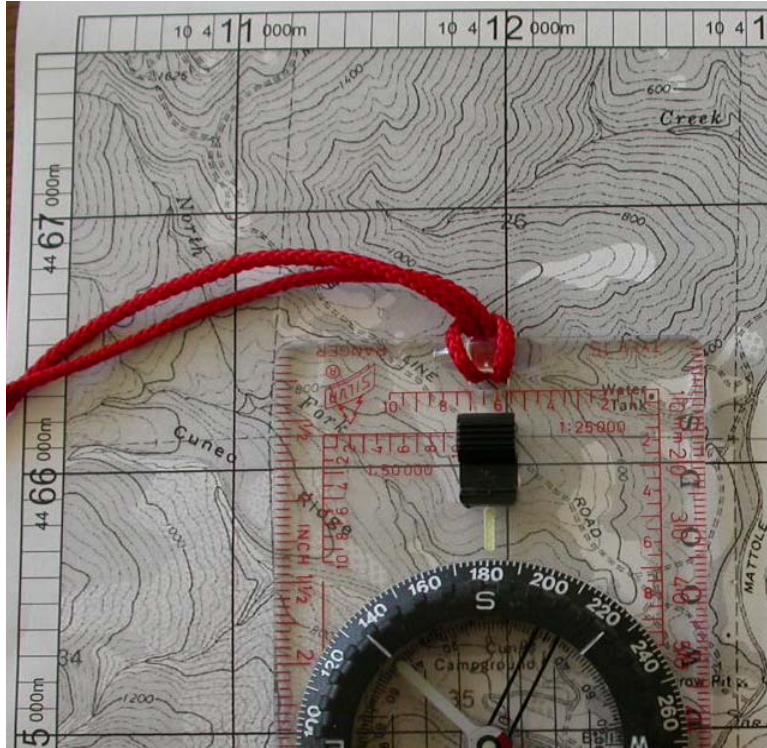
Figure 4. Use of “Roamer” Scale on Compass and UTM Grid on Map to Determine Coordinates of Water Tank.
