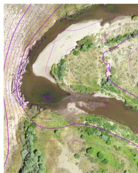
Elevation contours produced from drone-derived elevation model
