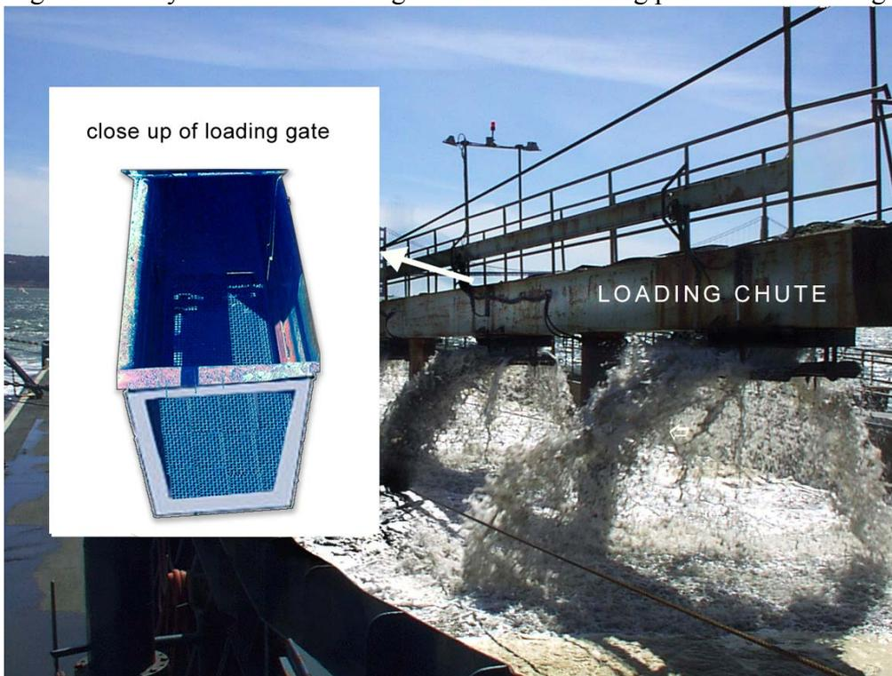
Figure 3-6. Barge loading chute and gate.
