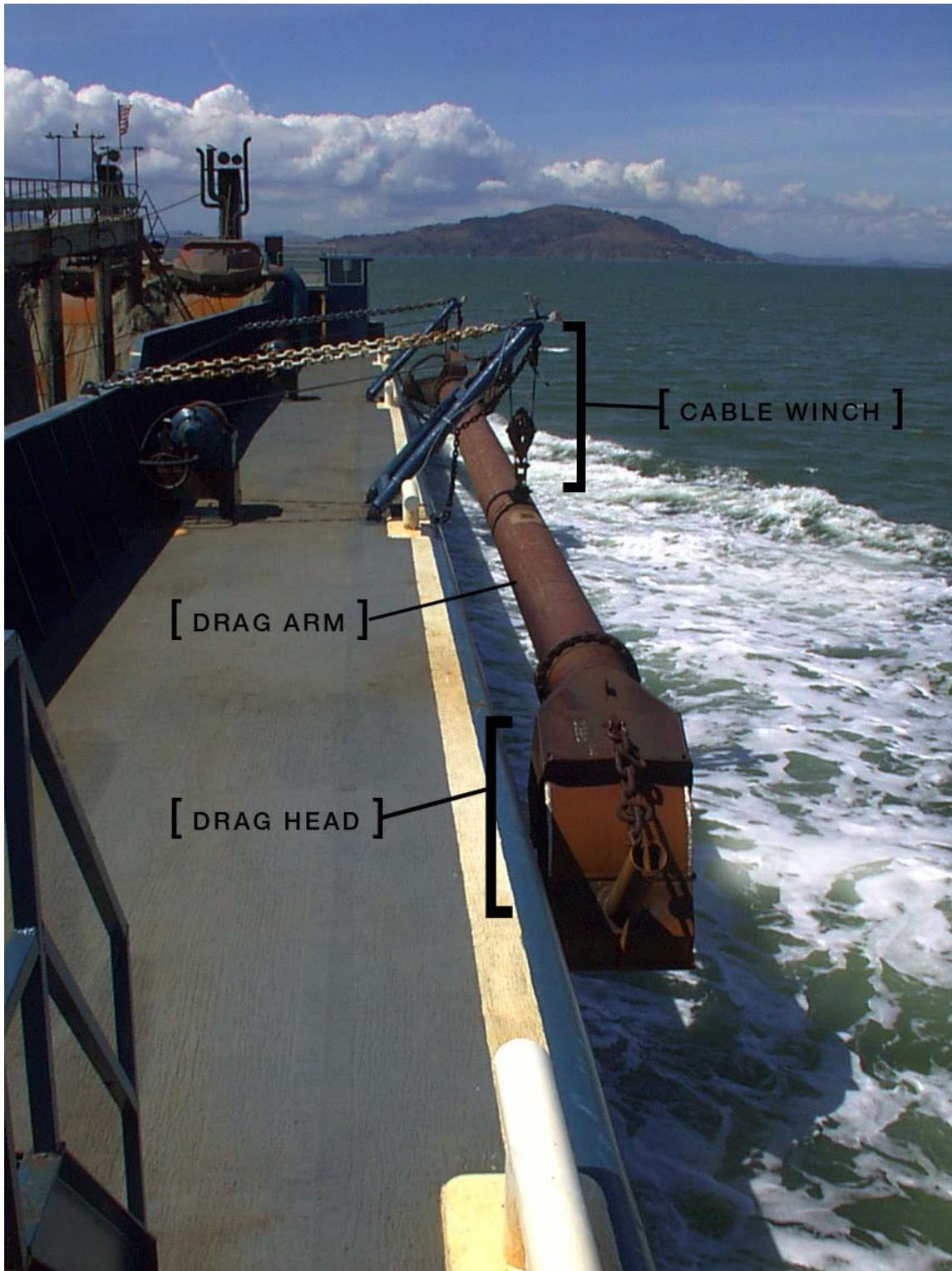
Figure 3-3a. Hydraulic suction drag arm and drag head assembly in the retracted position
