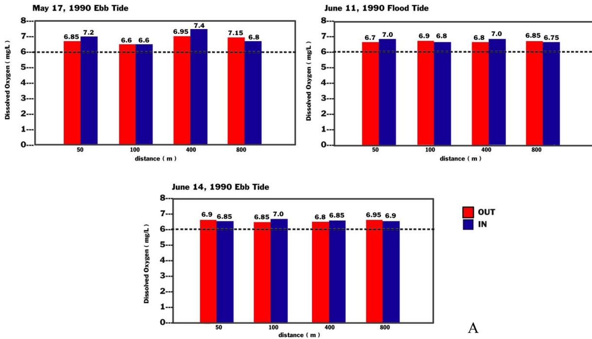
**Figure 5-4. Dissolved oxygen concentration at 20-foot depth inside and outside of an overflow plume during sand mining in Central Bay (MEC and Cheney 1990).**
