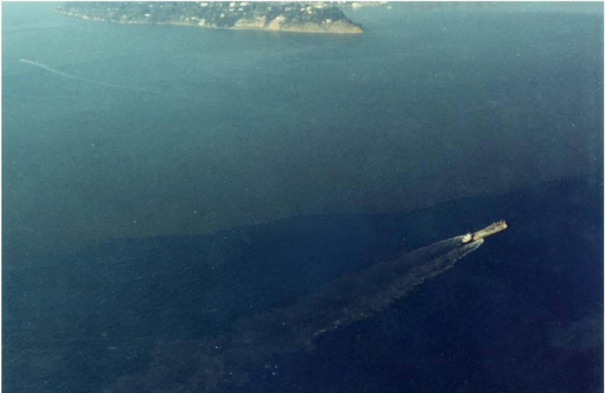
Figure 3-9. Sand mining overflow plume and natural turbidity at ebb tide within Central Bay
