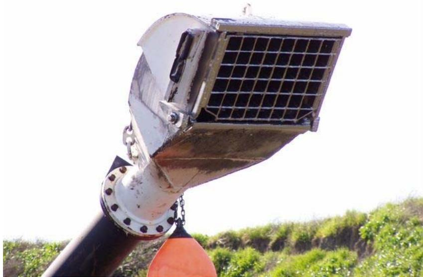
Figure 3-4. Hydraulic suction drag head showing “grizzly” screen used to exclude large material during sand mining.
