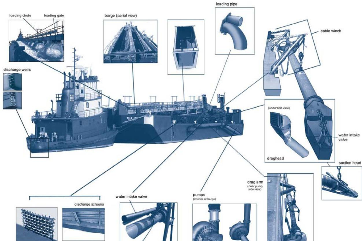
Figure 3-2. Schematic of typical sand mining barge
