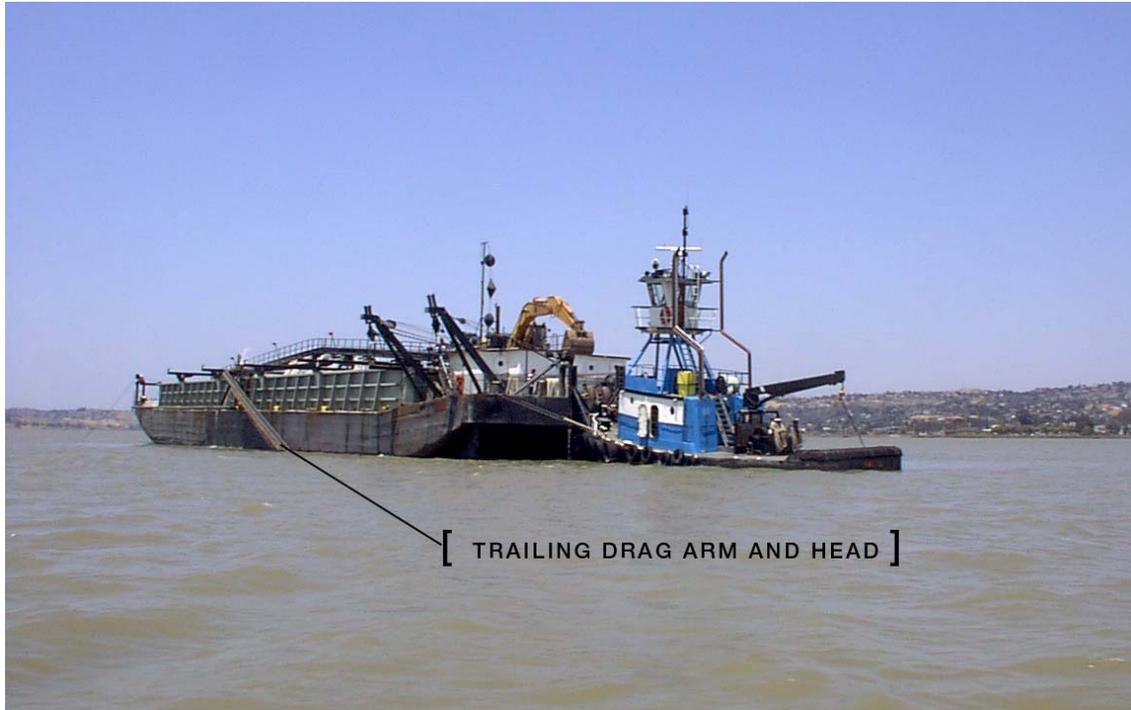
Figure 3-3b. Trailing drag arm and hydraulic suction drag head
