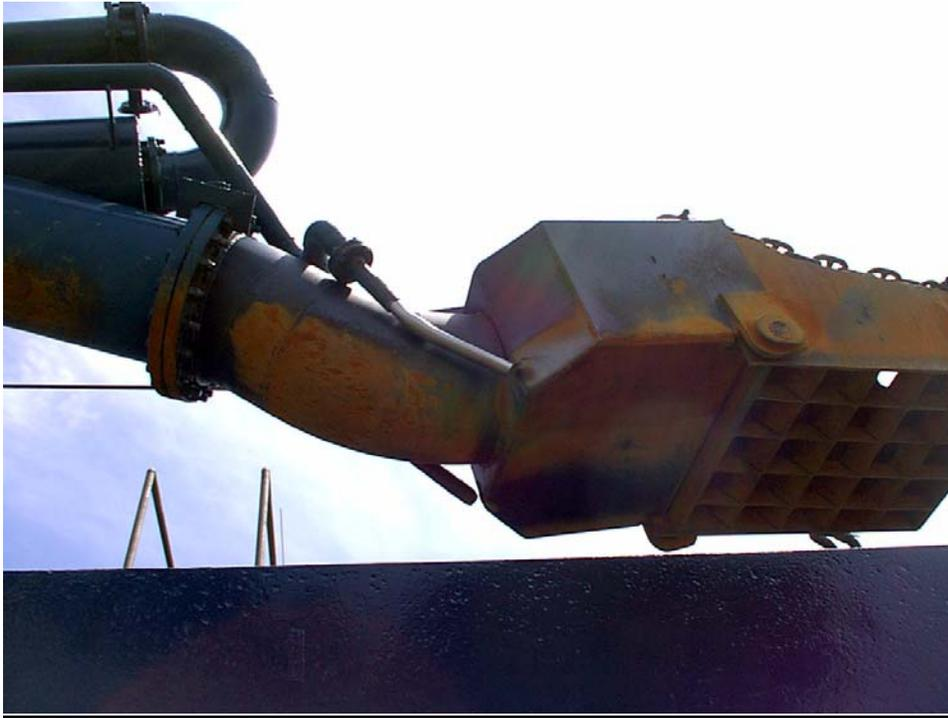
Figure 3-5. Hydraulic suction drag head used in moving pothole sand mining.
