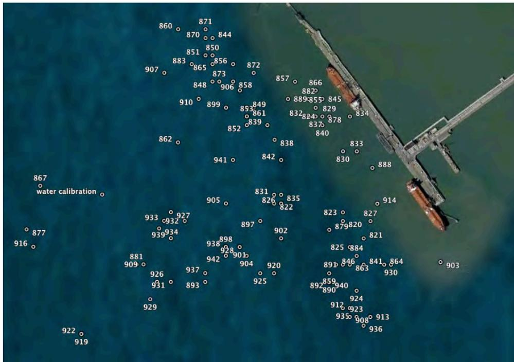
**Figure 4. Detailed Image of Hopper Loads Collected During Richmond Long Wharf Dredging Operations, July 19<sup>th</sup>, 2011 through July 31<sup>st</sup>, 2011.**
