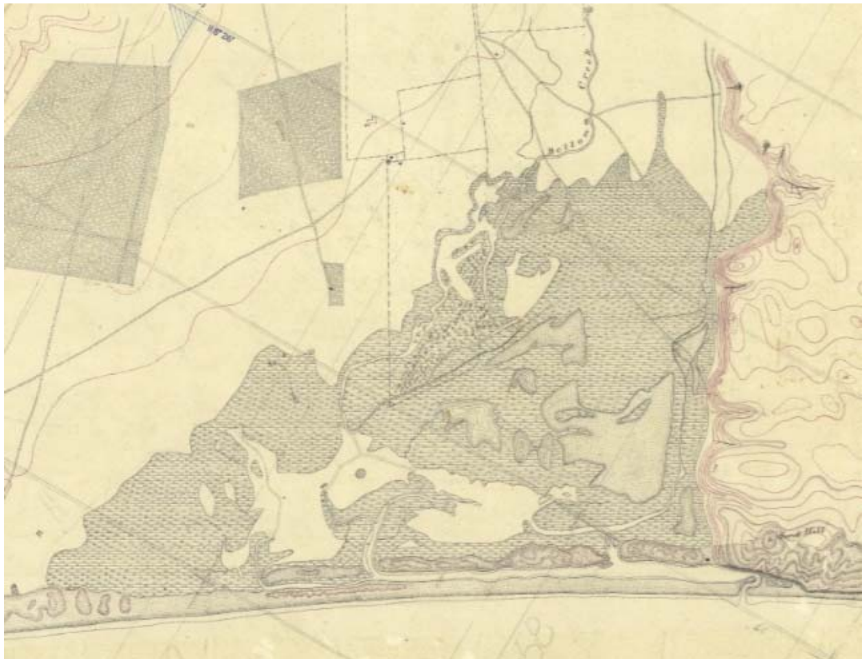
Figure 9. Detail of 1876 coast survey map (T-Sheet) of Santa Monica Bay. A small opening to the ocean is visible at the southern end of the dune system where it abuts the consolidated terrace.
