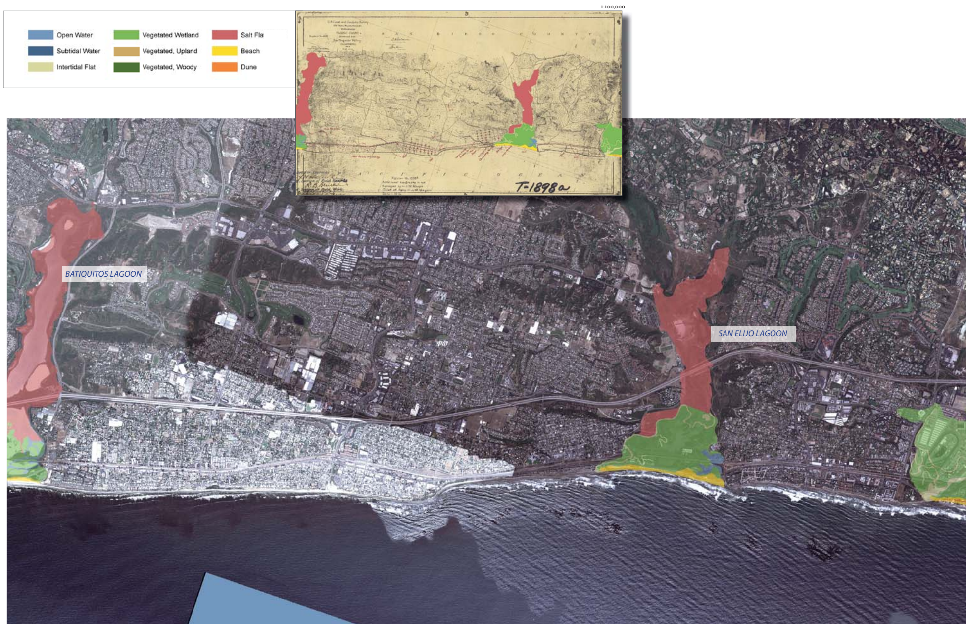
Figure 27. Coastal features digitized from T-1898, overlaid on modern aerial photography (USDA 2005), at same scale as facing T-sheet.
