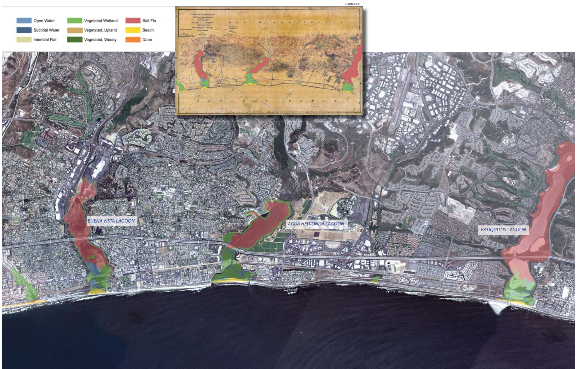
Figure 24. Coastal features digitized from T-1899, overlaid on modern aerial photography (USDA 2005), at same scale as facing T-sheet.
