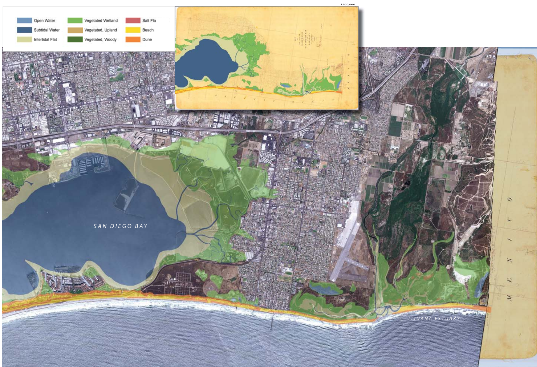
Figure 30. Coastal features digitized from T-365, overlaid on modern aerial photography (USDA 2005), at same scale as facing T-sheet.
